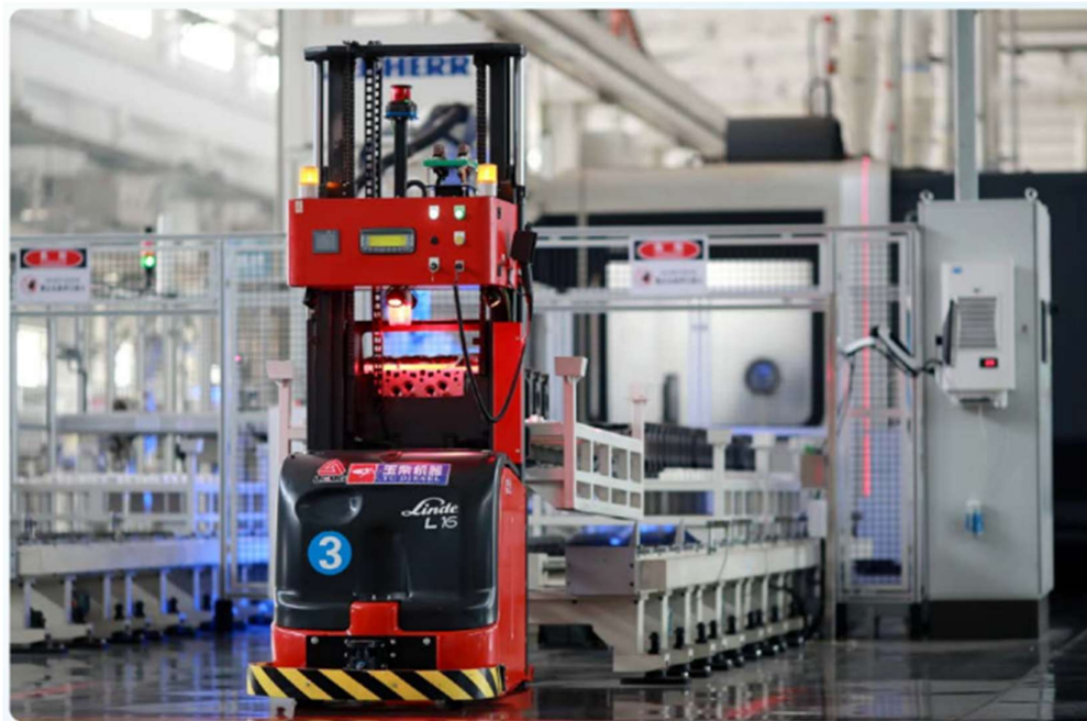
Figure 11: Yuchai's robotic automatic system, which includes automated loading and unloading robots handling cylinder head casting for machining processes
